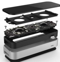
Figure 1: The representation of interior design of Leap Motion taken from its product page.
