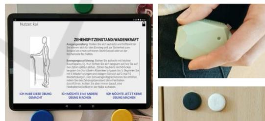
Figure 4: ActiConverge prototype (tablet-based PC with exercise program, Bluetooth beacon, Bluetooth buttons).
