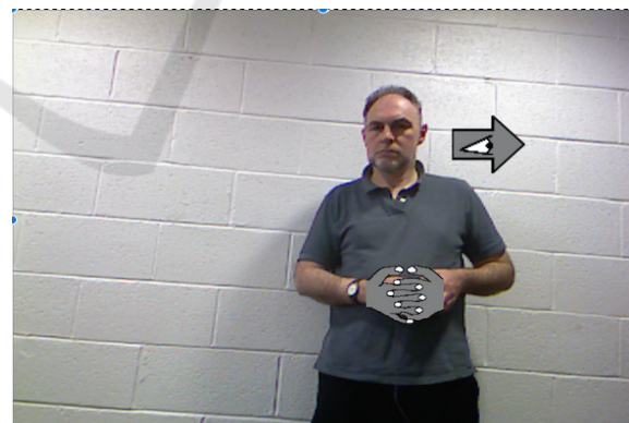
Figure 3: System Video Stream with visual feedback on gaze direction and hands-touching. The user is represented in the video.
