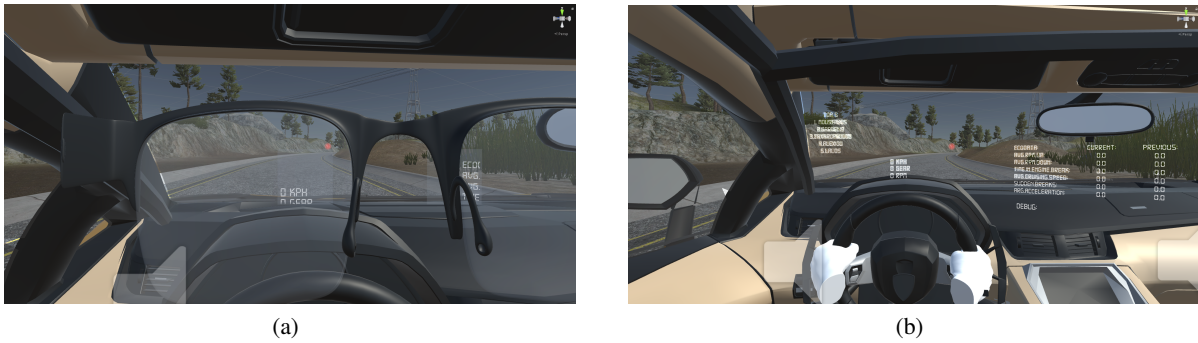
Figure 7: (a) Viewport window of the AR glasses (b) All the AR data that are being projected in the windshield.
