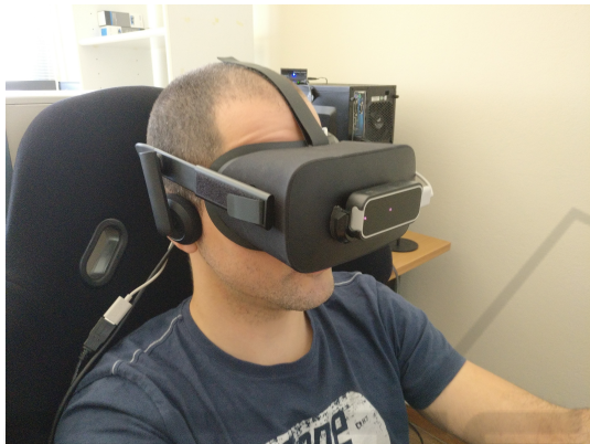
Figure 8: Leap motion sensor placed on Oculus Rift.
