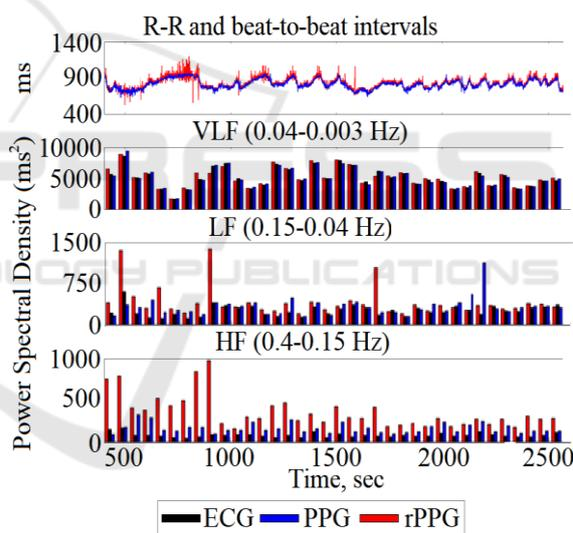
Figure 4: The example of power spectral density values of ECG, PPG and rPPG signals during the HFJV.
