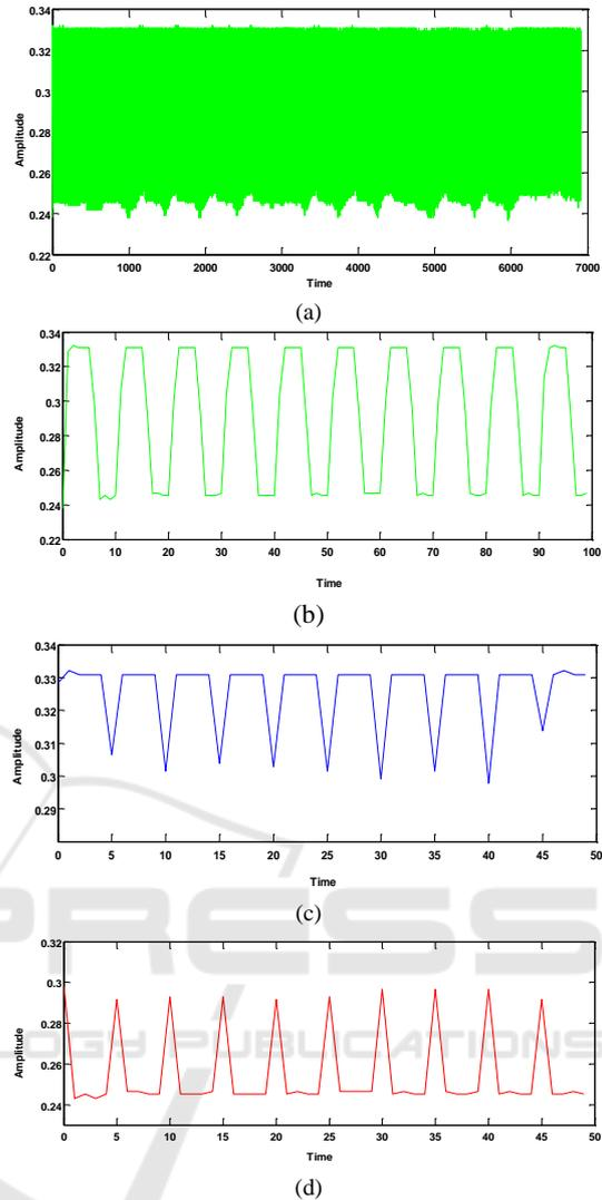
Figure 9: (a) Photodiode output signal in the third testing phantom: 2.5% of intralipid in 1% agarose solution, (b) First 100 sample points of recorded signal, (c) Upper amplitude variation in the signal which corresponded to on time period of LED source 850 nm, (d) Lower amplitude variation in the signal which corresponded to on time period of LED source 770 nm.
