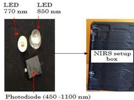
Figure 3: One channel NIRS setup.
