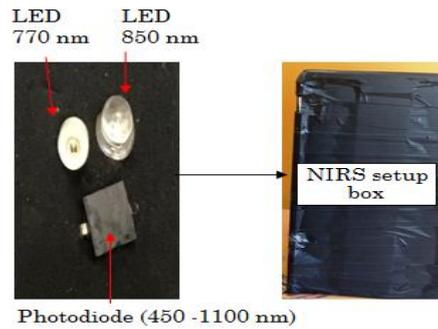
Figure 3: One channel NIRS setup.
