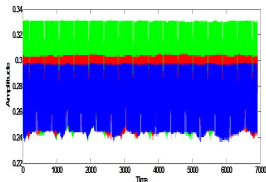
Figure 6: Photodetector output voltage for three test phantoms.
