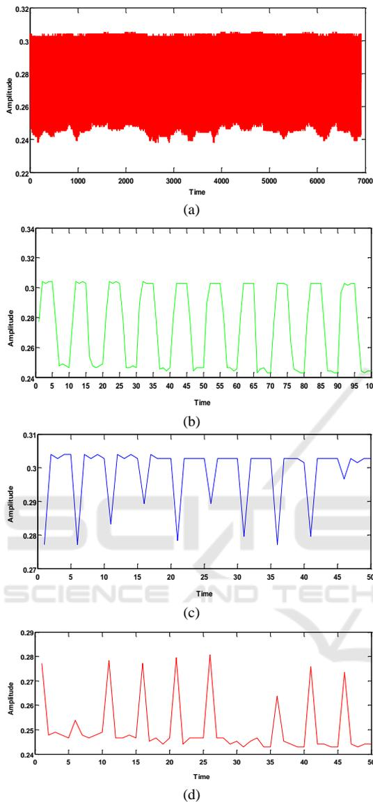
Figure 8: (a) Photodiode output signal in thesecond testing phantom: 1.25% of intralipid in 1% agarose solution, (b) First 100 sample points of recorded signal, (c) Upper amplitude variation in the signal which corresponded to on time period of LED source 850 nm, (d) Lower amplitude variation in the signal which corresponded to on time period of LED source 770 nm.
