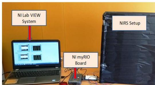
Figure 5: Experimental set-up for testing phantoms.
