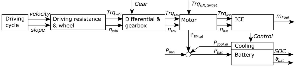
Figure 4: Signal flow diagram of the HEV model.
