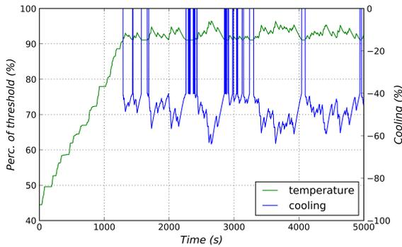
Figure 9: Battery temperature relative to the threshold for power limitation (green) together with the control of cooling power (blue) for simulative driving of a 5.000s long stochastic cycle based on NYCC with the operating strategy learned by the agent.
