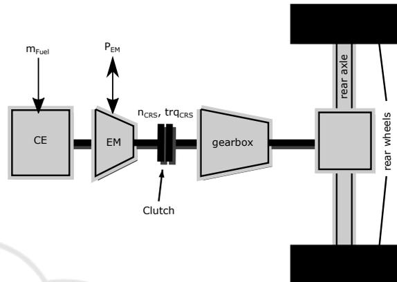
Figure 1: Structural scheme of a parallel mild hybrid.
