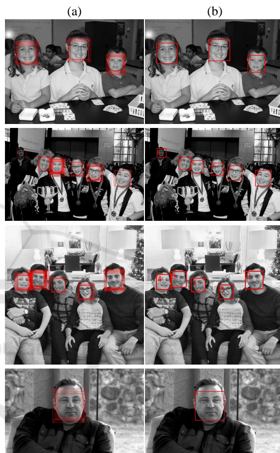
Figure 7: “Faces”: examples of correct detections by the best among detectors trained on statistical moments ( n = 3, N = 7, B = 16 ) — (a) direct outcomes with all single indications, (b) postprocessed outcomes after grouping clusters of windows.
