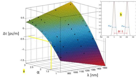
Figure 3: (a) 3-D plot showing which  $\alpha$  suits best for the mode separating fibre ( $\alpha = 1.6$ ), used at a specific wavelength, to reach a clear separation of the mode groups after travelling through the fibre (b).
