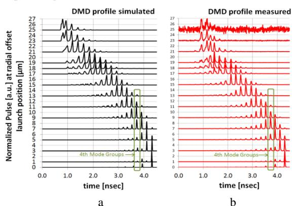
Figure 2: simulated and measured DMD profile after 550 m of the ‘ $\alpha = 1.6$  fibre’ (mode separating fibre). 18 Mode Groups are visible and clearly separated in time.
