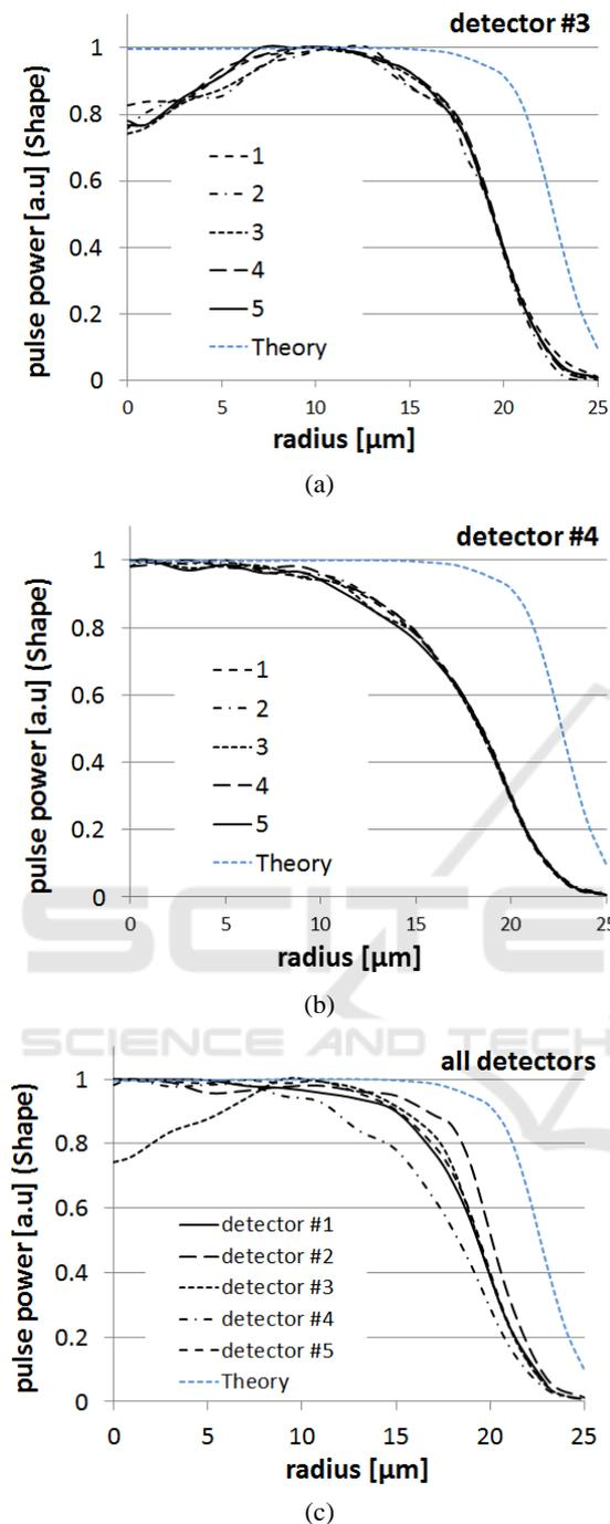
Figure 7: (a) reproducibility of detectors #3 and #4. (b) Shape of all five detectors.
