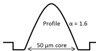
Figure 1: refractive index profile of the special designed fibre (‘mode separating fibre’).
