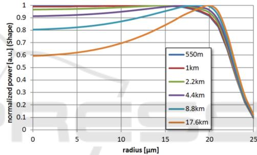
Figure 4: Theoretical power distribution ('Shape') over a Graded Index 50  $\mu\text{m}$  core fibre. The distribution changes with fibre length.
