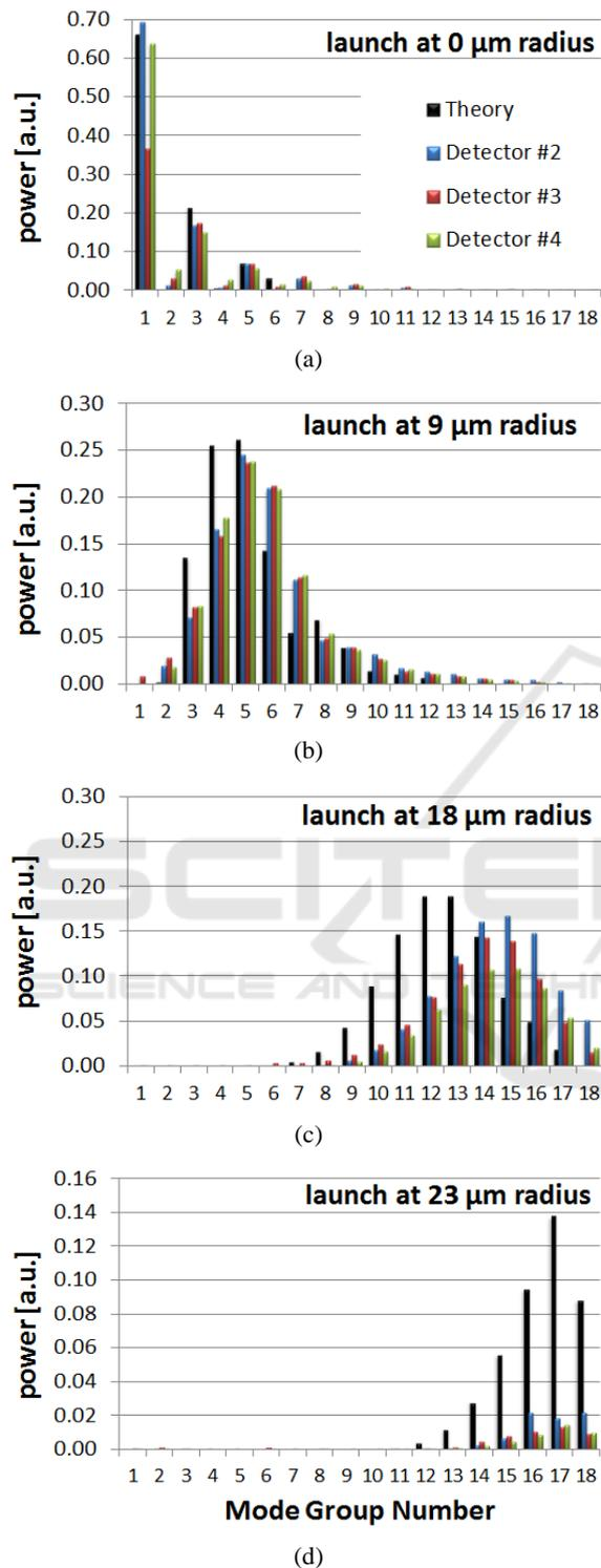
Figure 8: Detected mode group powers of the #3 detectors considered at launch radii of 0 μm (centre), 9 μm (most mode groups detected), 18 μm (relevant for ‘inner’ DMD), and 23 μm (‘outer’ DMD).
