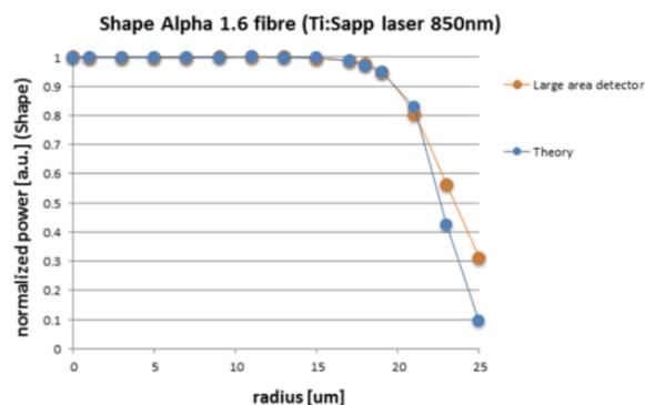
Figure 6: theoretical and verified 'DC' power distribution (Shape) after 550 m  $\alpha = 1.6$  fibre.
