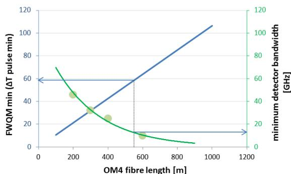
Figure 5: laser pulse and detector requirements to qualify OM4 fibre at different lengths.
