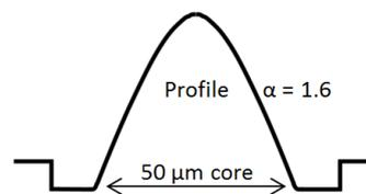
Figure 1: refractive index profile of the special designed fibre (‘mode separating fibre’).
