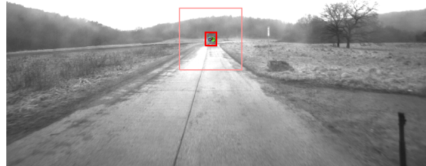
(a) Long range markerless tracking. The tracked vehicle is marked with a red bounding box.
