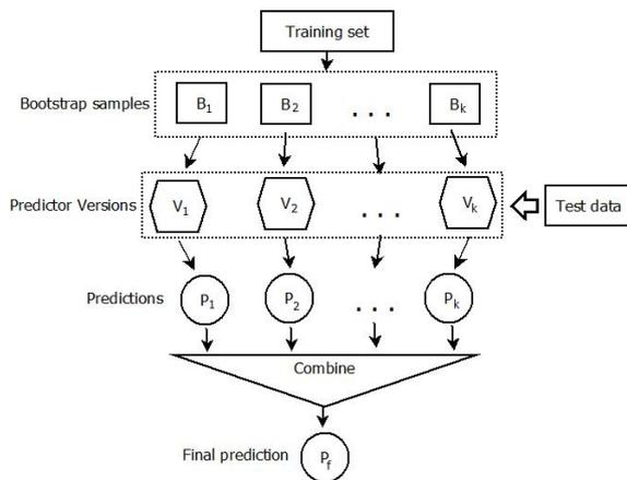
Figure 2: Summary of the process of bagging. From the training set,  $k$  bootstraps are created. Each bootstrap  $B_1, \dots, B_k$  is used to build predictor versions  $V_1, \dots, V_k$  which make separate predictions  $P_1, \dots, P_k$ . The final prediction  $P_f$  is a combination (average for regression, majority voting for classification) of all the predictions.
