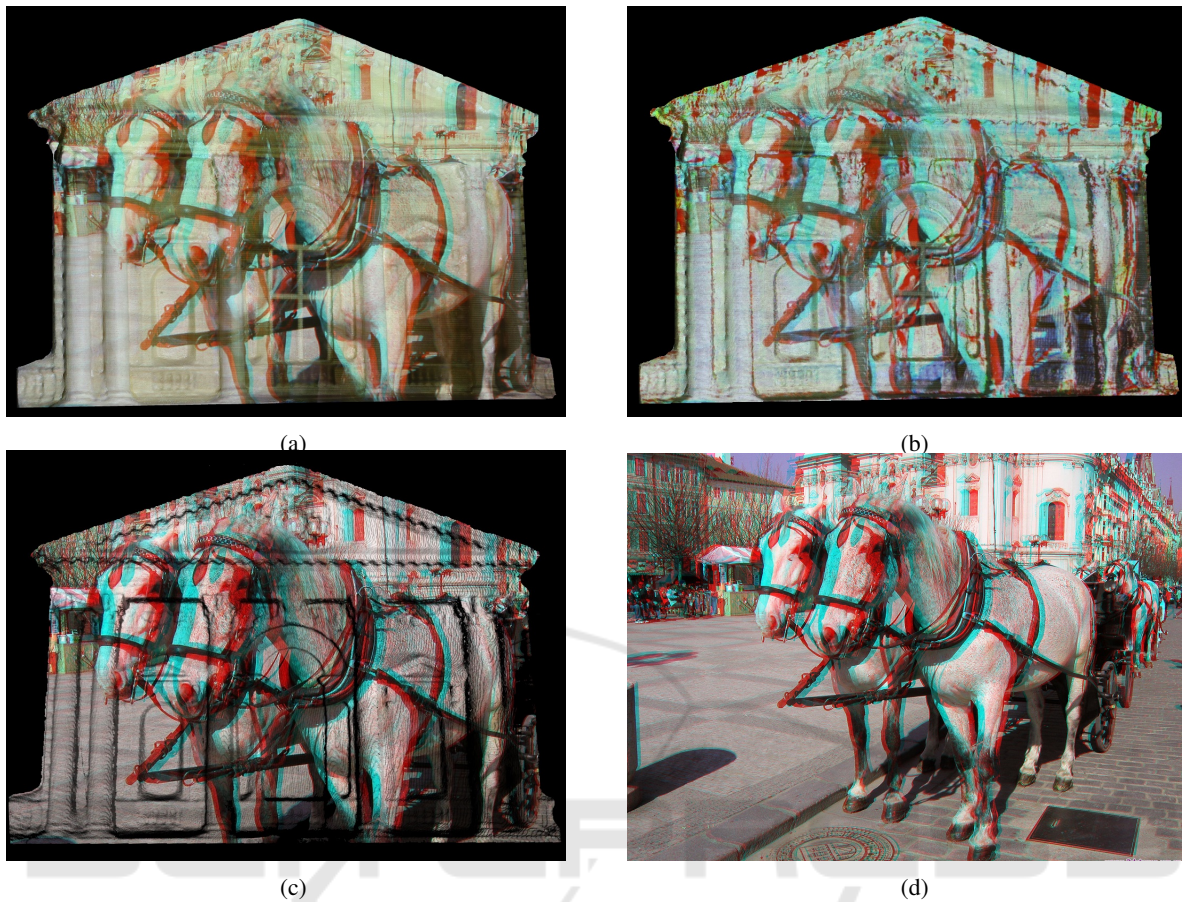
Figure 7: (a) A stereoscopic projection without compensation. Color distortions due to the reflectance properties of the projection surface negatively affect the depth perception of the viewer. (b) The stereoscopic projection after compensation using the proposed technique. Color distortions are minimized by taking into account the effect of the reflectance properties of the projection surface. (c) The expected projection. This cannot always be achieved due to the limitations of additive color mixing and the hardware. (d) The original stereoscopic image taken from (ste, ).
