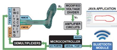
Figure 1: Block diagram of the system.
