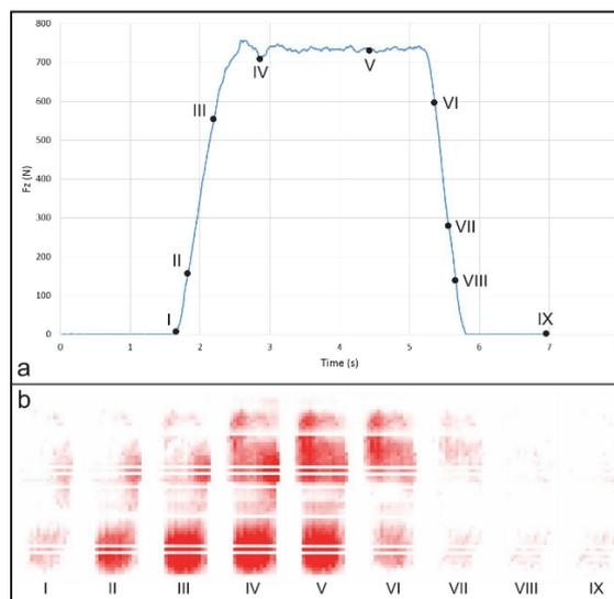
Figure 12: Load transfer from the left lower limb to the right: a) Force measured by Biomechanics Platform; b) Plantar pressure detected by the wearable device.
