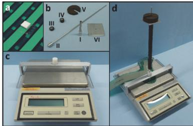
Figure 3: a) Load actuator fixed on SE; b) I - shaft, II - support of loads, III - 5g block, IV - 10g block, V - 100g block, VI - support plate; c) Custom built structure in weight scale; d) All loads applied to the SE; sensor fixed on weight scale plate.
