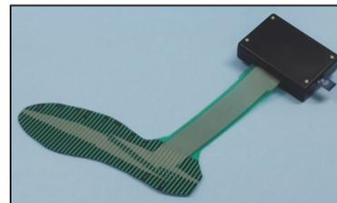
Figure 9: Wearable device: data acquisition module and Medical Sensor 3000 (215g).
