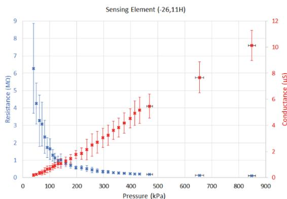
Figure 8: Characterization of SE in relation to applied pressure and  $R_s$  and  $C_s$ .
