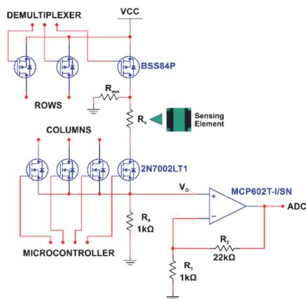
Figure 4: Schematic of data acquisition circuit, including switching circuit to select each SE. Whole circuit has eight sets with four NMOS and one operational amplifier.
