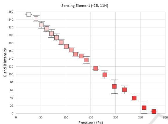
Figure 11: Color of graphic element according to the employed pressure. Mean and SD were approximated to integer values.
