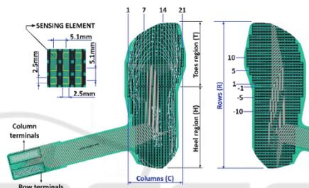
Figure 2: Bottom and top views of Medical Sensor 3000.
