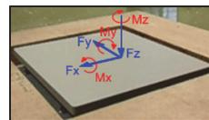
Figure 5: Biomechanics Platform – sign convention for the force and moment components defined by AMTI.
