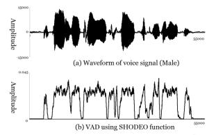
Figure 3: Comparison among VAD methods in word (male) (a) waveform of voice signal (b) VAD using SHODEO function.
