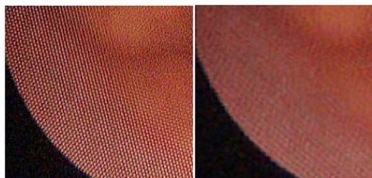
Figure 3: Left- cropped section of original RGB image to illustrate the honey-comb structured artefact caused by the fibre-optic bundle; Right: pre-processed image with artefact suppressed.
