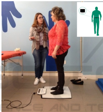
Figure 1: Example of a test set-up, with the pressure platform in the floor and an illustration of the inertial sensor placement of at the lower back, since it is covered by the clothes.
