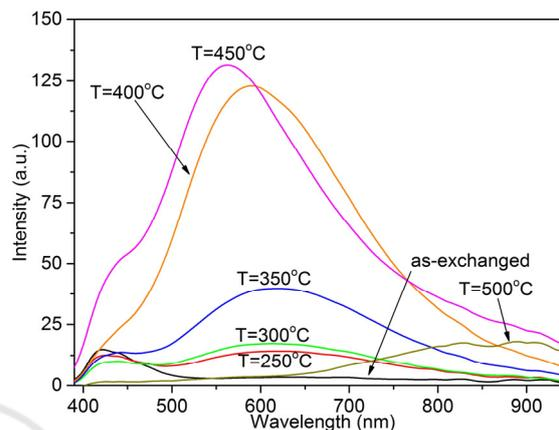
Figure 3: Emission spectra ( $\lambda_{ex} = 365$  nm) of the ion-exchanged PTR matrix-based glass GS10 prior to any heat treatment and after the heat treatment at temperatures 250-500 °C (temperature values are indicated on the graph).
