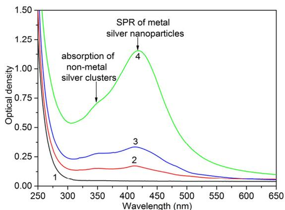
Figure 1: Optical density spectra of PTR glasses GS0-GS10 (1)-(4), respectively, after the IE and subsequent heat treatment at 500 °C.
