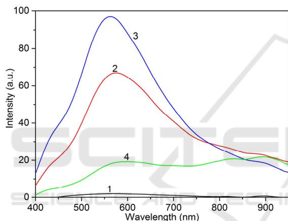
Figure 2: Emission spectra ( $\lambda_{ex} = 365$  nm) of PTR glasses GS0-GS10 (1)-(4), respectively, after the IE and subsequent heat treatment at 500 °C.
