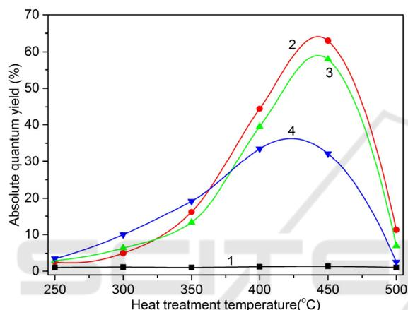
Figure 5: Dependence of AQY magnitudes for ion-exchanged PTR glasses GS0-GS10 (1)-(4), respectively, on the temperature of the subsequent heat treatment.
