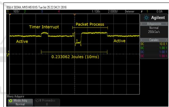
Figure 11: Characteristic of AM Packet.
