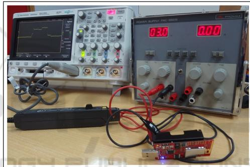
Figure 5: Measurement set-up: Power supply and oscilloscope connected to the transmitter.
