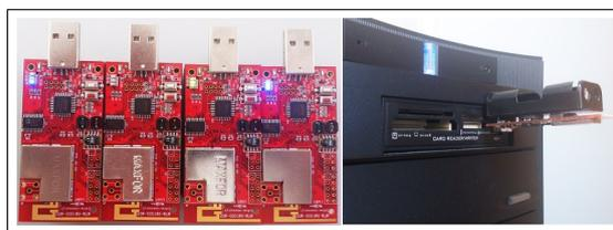
Figure 1: Model of testbed used in the performance evaluation, XM1000 (Advanticsys), and one coordinator connected to USB port.
