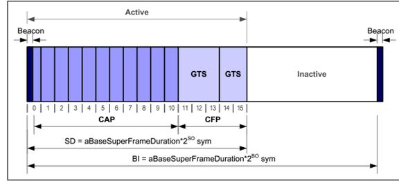
Figure 4: Superframe Structure with BO and SO parameters.
