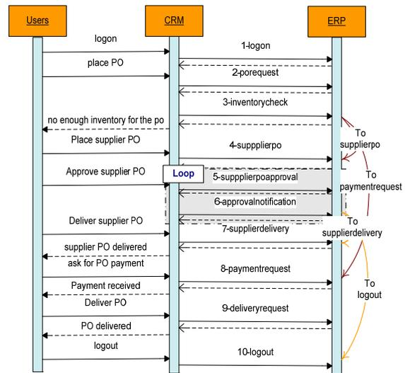
Figure 1: A CRM and an ERP sales process flow diagram.
