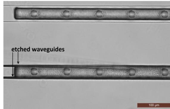
Figure 14: Top view of the optofluidic device.
