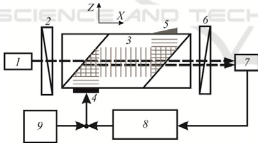
Figure 4: AO spectrum analyzer scheme.
