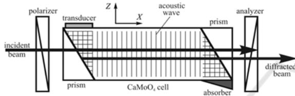
Figure 1: Collinear AO filter scheme.
