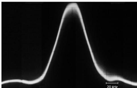
Figure 2: Transmission function of conventional collinear AO filter.
