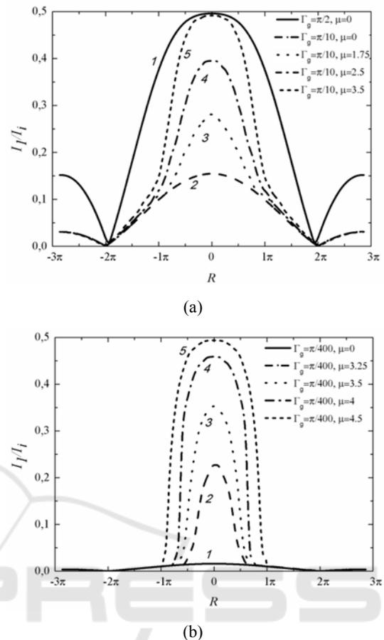
Figure 6: AO collinear cell with feedback circuit transmission functions. a – Raman-Nath parameter  $\Gamma_g = \pi/10$ . b -  $\Gamma_g = \pi/400$ .
