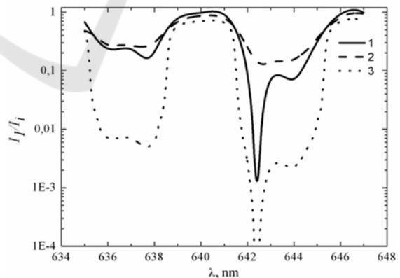
Figure 10: AO optical spectrum analyzer operation. Curve 1 - spectrum on the input  $I_i(\lambda)$ , curve 2 - light spectrum on the output of conventional collinear AO filter  $\Gamma = \pi$ , curve 3 - light spectrum on the output of AO system with feedback  $\Gamma_g = \pi/100$ ,  $\mu = 5.5$ .
