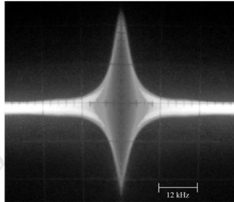
Figure 5: AO filter transmission function with feedback.
