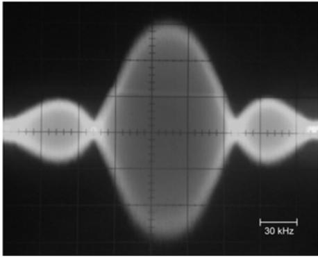
Figure 3: AO collinear filter transmission function for  $I_1$  component.
