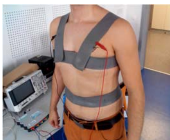
Figure 6: Measurement of one-lead ECG on chest with using of strap.
