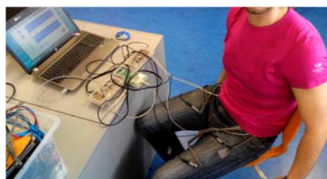
Figure 15: Measuring chain for measuring one-lead ECG from T-shirt by PPy cotton electrodes with PANI carbon conductors and in the same time by stick Ag/AgCl electrodes (placed on the human body) with common wires.
