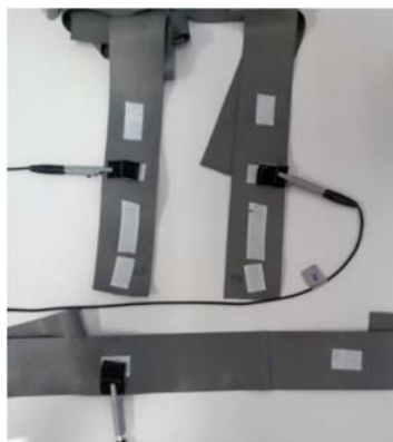
Figure 5: Strap with PPy electrodes connected by conductors.
