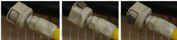
Figure 7: A variety of reference images of the same adapter because of the longitudinal rotations, which are not detectable with the feature detection algorithms.
