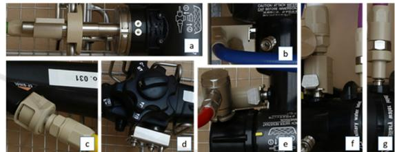
Figure 9: Adapter set which we used for our experiments.
