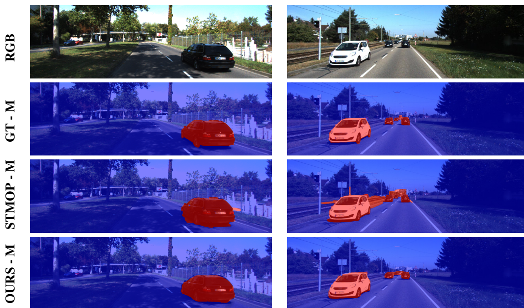
Figure 6: Qualitative evaluation - Motion segmentation on our KITTI test dataset. On the left, the images, consist of single moving car. On the contrary, we have multiple cars in the image, on the right. Blue pixels represent stationary and red pixels depict motion. We compare our approach with STMOP-M moving object proposals (Fragkiadaki et al., 2015). In the figure, GT - M is ground truth motion annotation, STMOP - M is output from (Fragkiadaki et al., 2015) and OURS - M is the motion segmentation obtained from the proposed approach. In contrast to STMOP-M where over-segmentation and False Positive cases are observed on the roads and fence, our proposed approach yields better segmentation and motion boundaries with cars in motion. (Best viewed in color).
