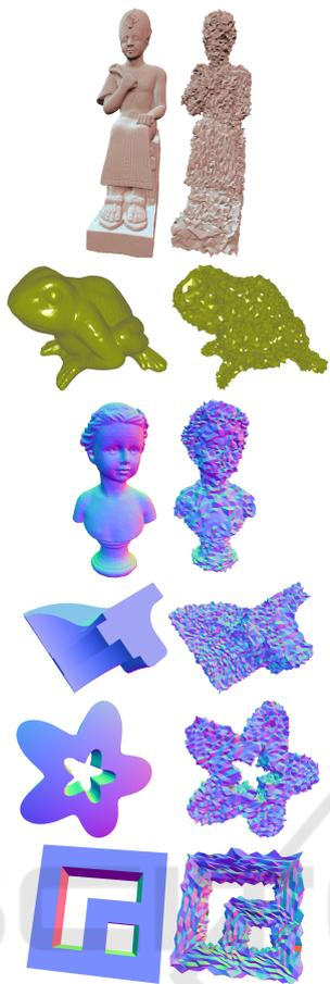
Figure 2: Mesh models with added uniform noise (vertex displacements half the mean edge length).
