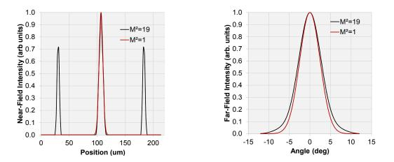
Figure 9: Near-field (left) and far-field (right) intensity distributions of an engineered structure operating with  $M^2$  of 19 and 89% of its power in the far-field within the diffraction limit.
