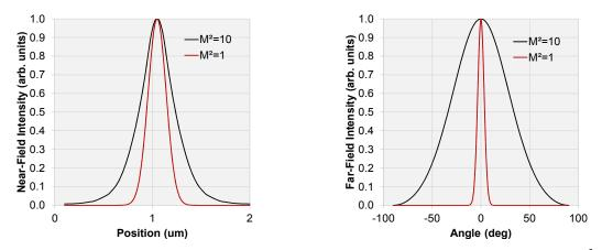
Figure 7: Near-field (left) and far-field (right) intensity distributions of an engineered structure operating with  $M^2$  of 10 and only 20% of its power in the far-field within the diffraction limit.
