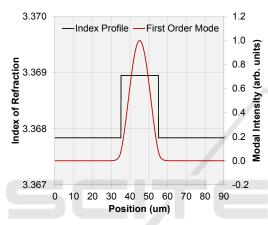
Figure 1: A basic refractive index structure and its first order mode profile. Note that many higher order modes are also supported by this structure.
