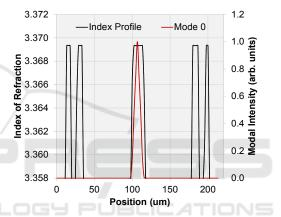
Figure 8: The index profile and first order mode of the engineered structure that supports the original hypothesis.
