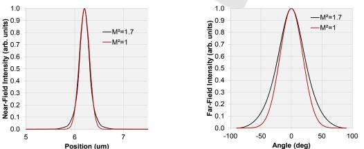
Figure 6: Near-field (left) and far-field (right) intensity distributions for an engineered structure with M<sup>2</sup> of 1.7 and 86 percent of its power in the far-field within the diffraction limit.
