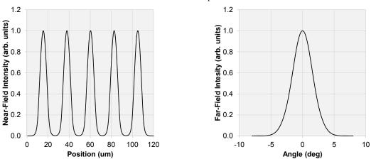
Figure 5: The near-field (left) and far-field (right) intensity profiles for the structure in Fig. 2.
