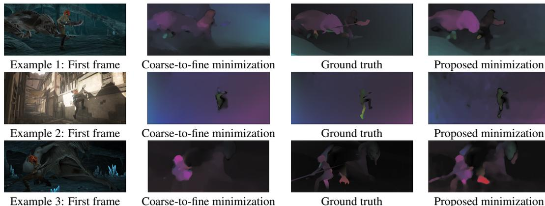
Figure 3: Comparison of two minimization strategies for the same energy proposed in (Wedel et al., 2011). Our minimization strategy is not based on a coarse-to-fine scheme but on sparse correspondences that allow to capture large displacements. Results in the MPI Sintel training set.
