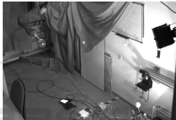
Figure 2: The Throwing-and-Catching test environment consists in a robot arm, multiple LED floodlights, two parallel aligned cameras, and a throwing device that accelerates a tennis ball to overcome the distance of about 2.5m.
