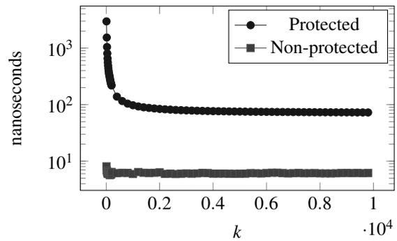
Figure 4: Execution time of Algorithm 1 in nanoseconds. The figure presents two graphs that correspond to two execution modes: (1) protected mode, in which the algorithm is realized by an encrypted method, (2) non-protected mode, in which the algorithm is realized by a regular, non-encrypted method.
