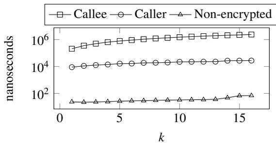
Figure 5: Execution time of Algorithm 2 in nanoseconds. The figure presents three graphs that correspond to three execution modes: (1) the callee, i.e. the function  $f_k$ , is encrypted (2) the caller is encrypted (3) neither the caller nor the callee are encrypted.
