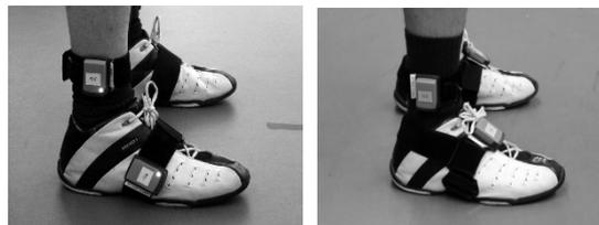
Figure 1: Two placements of foot sensors (on the side – left, on the top of the foot - right).
