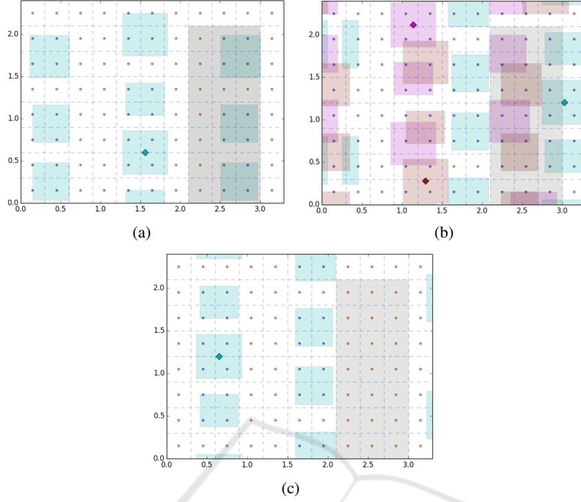
Figure 2: Three deployments scenarios considered during the experimentation. Circle points represent the discrete grid of the deployment area and diamond points represent the PIRs. The gray zone delimits the place of the office’s desk, which has been given a greater weight in  $\Phi$ . (a) Optimal deployment with one PIR. (b) Optimal deployment with three PIRs ensuring full coverage of the desk’s area. (c) Hole-unaware deployment where the desk area is completely uncovered.
