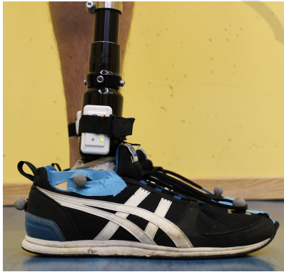
Figure 1: Marker and sensor placement on the amputated leg.
