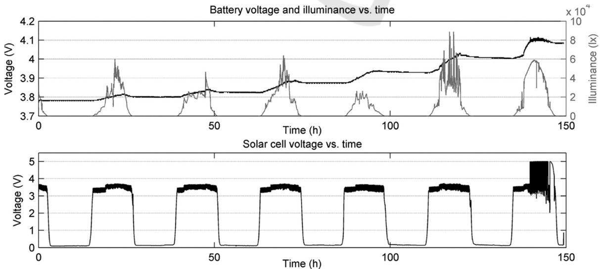
Figure 5: Energy harvester performance over six days.
