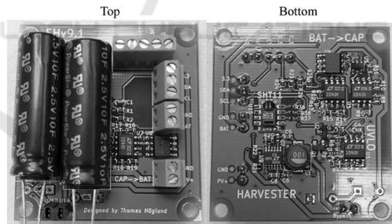
Figure 2: Developed energy harvester prototype.
