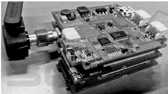
Figure 1: The UWASA Node with power module.
