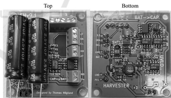
Figure 2: Developed energy harvester prototype.
