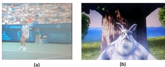
Figure 11: Attacked video watermarked (Chan and Lyu, 2003): (a) camcordered video with camera in the left of the screen + deformation + compression 500 kbit/s, (b) camcordered video with camera down of the screen + deformation + compression 500 kbit/s + Cropping.
