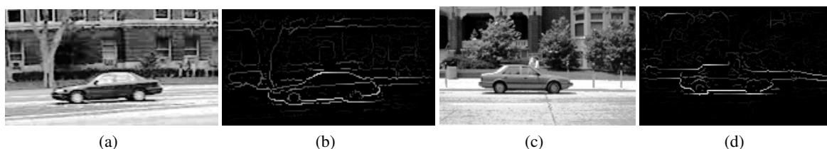
Figure 2: (a) Input image (b) Output of Structured Edge Detector (c) Input image (d) Output of Structured Edge Detector (both trained for car edge detection + sharpening).
