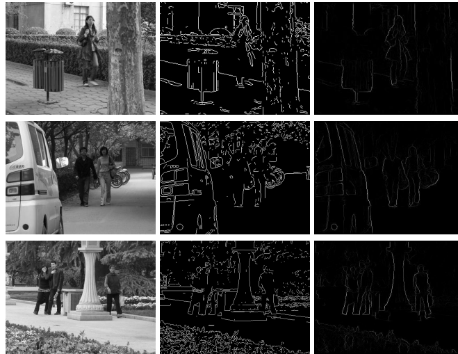
Figure 3: Examples of confusing Canny edges and background clutter in pedestrian localization. (Left) Input image (middle) Canny edge image (right) Output of Structured Edge Detector (trained for ped. edge detection).
