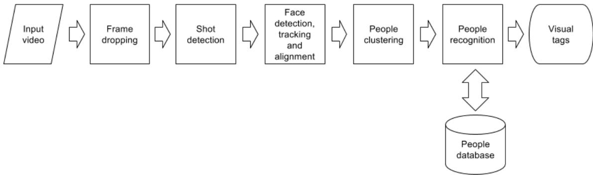
Figure 3: Schema of our visual indexing system.
