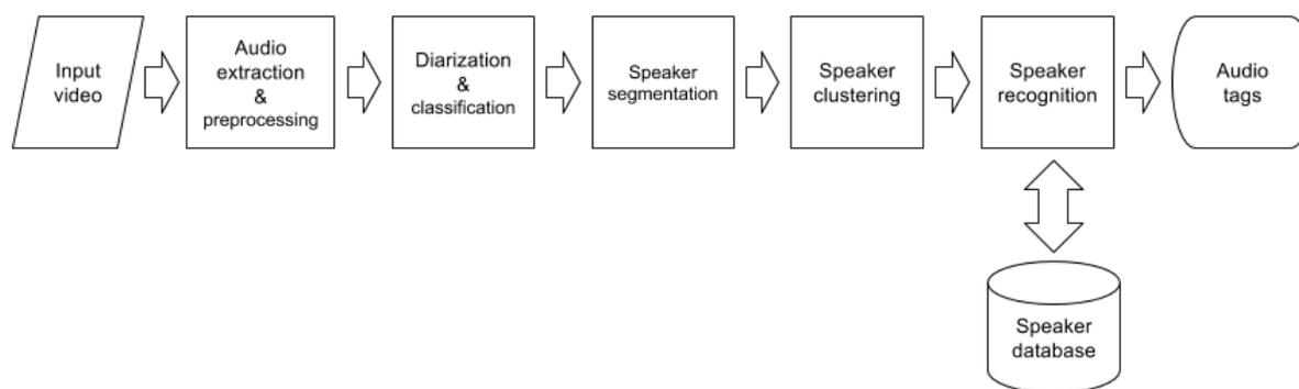
Figure 6: Schema of our audio indexing system.
