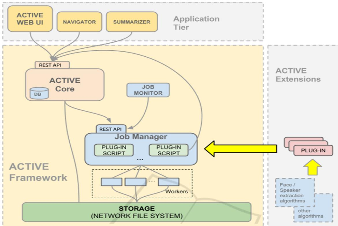
Figure 1: Schema of the ACTIVE System architecture.
