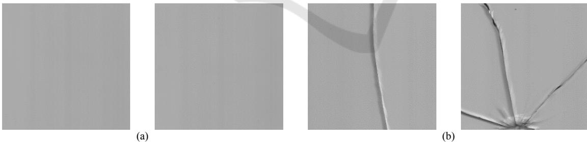
Figure 3: Glass sheet samples: (a) defect-free images; (b) defective images.
