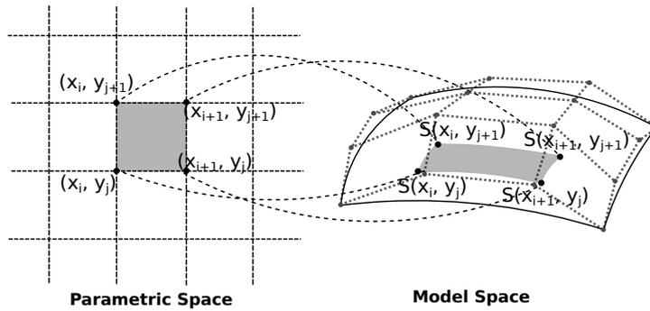
Figure 3: KSQuad primitive defined by a knot interval.
