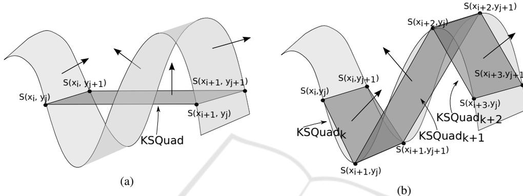
Figure 5: KSQuad-based culling (a) high degree NURBS (b) low degree NURBS.
