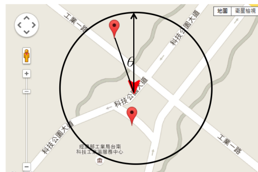
Figure 5: The camera heading angle between the current location and the marker.
