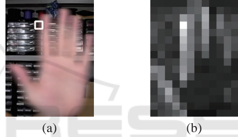
Figure 4: Example of a self similarity map using gradient intensity distributions. (a) Integrated gesture image I_{\text{intg}} ; (b) Computed self-similarity s_{\text{grad}}^{m',n} . The white block in (a) denotes the m' -th patch (the patch of interest).
