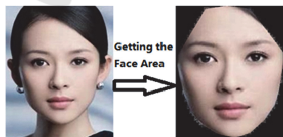
Figure 2: The process to locate the face region.
