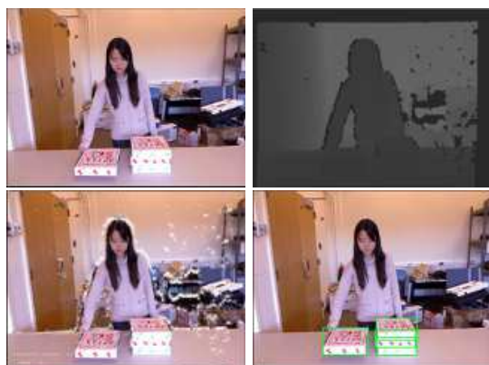
Figure 1: Multimodal database CAD120 with RGB (top left), Depth map (top right), 3D map (bottom left), object context (bottom right).
