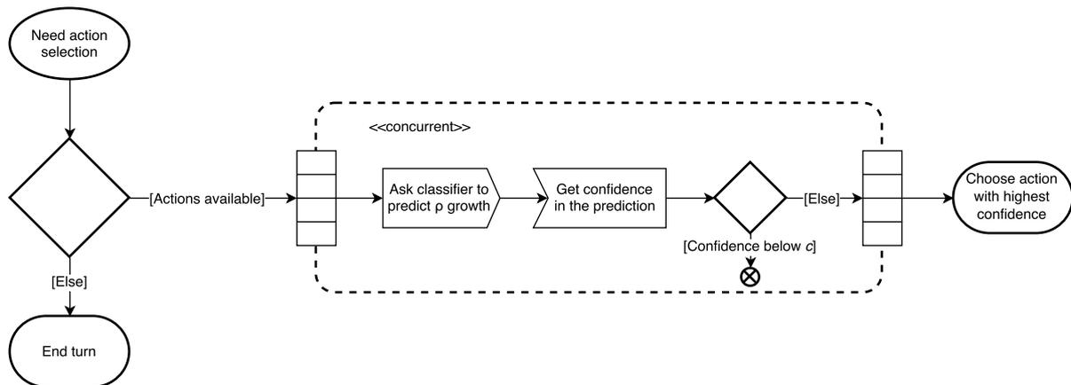
Figure 1: The action selection process.
