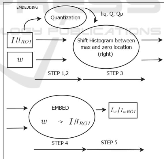
Figure 3: Embedding - block diagram.
