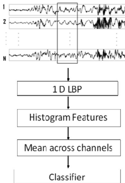
Figure 4: Schematic of the EEG classification system.
