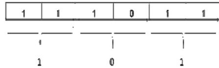
Figure 5: Post processing scheme for 2-minute window: Two consecutive ‘1’ labels give a ‘1’ in the output.
