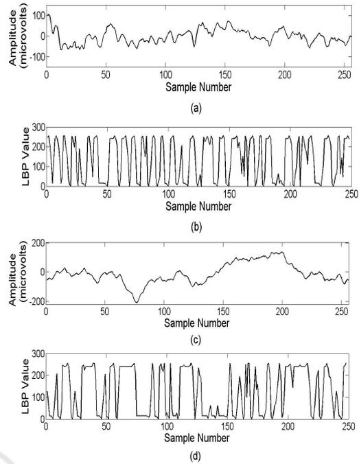
Figure 3: (a) A 1-second segment of interictal EEG signals of patient 1. (b) Interictal signal transformed to LBP domain, which has values ranging from 0 to 255. (c) A 1-second segment of preictal EEG signal from the first seizure of patient 1. (d) Preictal signal transformed to LBP domain.
