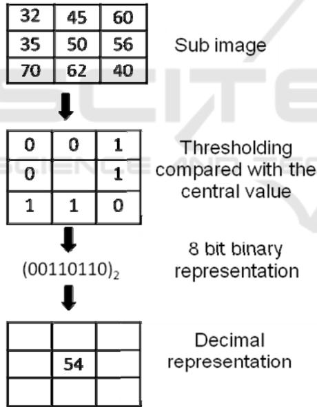
Figure 1: Calculation of LBP codes for a 3x3 sample block.  $P=8$ ,  $R=1$ .
