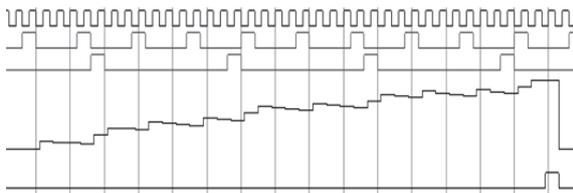
Figure 6: Simulation results of the Leaky Integrate and Fire model on Mentor Graphics Questa Sim 10.1d. Note: the first row is the biological clock, rows 2 and 3 represent synaptic inputs, row 4 is the neuron membrane voltage and row 5 represents the output spikes of the neuron.
