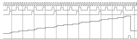
Figure 5: Simulation results of the Integrate and Fire neuron model on Mentor Graphics Questa Sim 10.1d. Note: the first row is the biological clock, rows 2 and 3 represent synaptic inputs, row 4 represents the neuron membrane voltage and row 5 represents the output spikes of the neuron.
