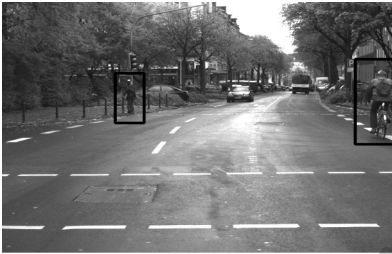
Figure 16: True Positive of pedestrian detection using the proposed method (black box: detection result).
