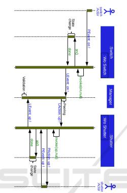
Figure 7: UML Sequence diagram of the interaction between a physical switch and a physical shutter.
