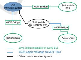
Figure 13: An IoT object, like a switch can be connected to WOF according to 3 ways: a) the thing can communicate using our MQTT protocol and its avatar exists in the WOF, b) the thing can communicate using our MQTT protocol but its avatar does not exist in the WOF, c) the thing cannot communicate using our MQTT protocol.
