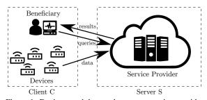
Figure 1: Devices send data to the remote service provider (server S) for storage and processing. The beneficiary, which resides on the client side, receives the processing results, either periodically or upon issuing a specific query.
