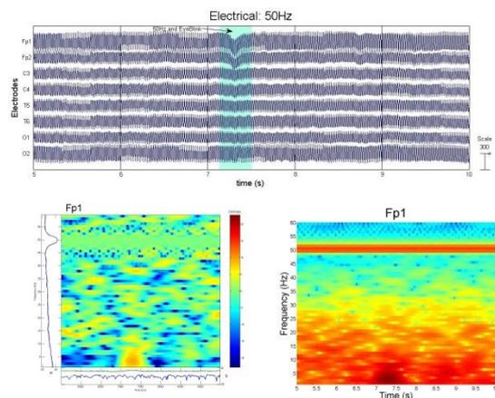
Figure 12: Electrical Artefact: 50Hz (Plot, ERSP, and Spectrogram).
