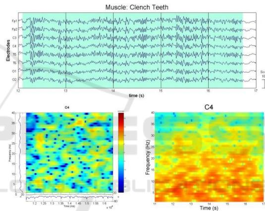
Figure 9: Muscle Artefact – Clench Teeth (Plot, ERSP, and Spectrogram).
