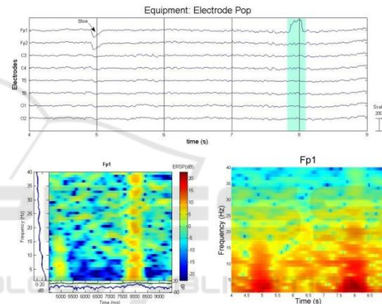
Figure 13: Equipment Artefact: Electrode Pop (Plot, ERSP, and Spectrogram).
