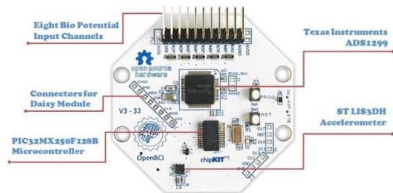
Figure 2: OpenBCI Board Components.
